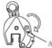
2. Place the clamp securely on the plate so that the jaw of the clamp rests on the plate (E).
