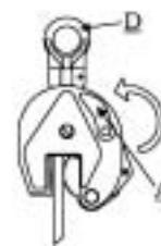
4. As soon as the load is at its destination let the crane hook descend until the clamp is fully free of load, meaning that the lifting chain is no longer taut and the hoisting eye (D) of the clamp can move freely. Now pull the safety latch (A) towards the jaw, allowing the clamp to be and remain opened.
