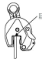
3. Now pull the safety latch (A) towards the hoisting eye (D). The clamp will now close and will remain on the plate in pretensioned position, allowing lifting to commence.
