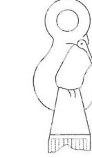
Figure 0.1 - Illustration showing inadequate accommodation of a wobbling eye. Or a hook of too small radius
